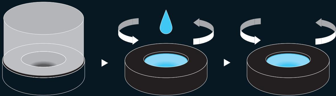
Spin casting molds are created for each contact lens specification
